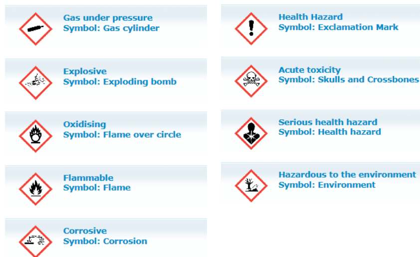
Figure 2: Hazard Classes and Pictograms for dangerous substances (CLP Regulation 1272/2008/Globally Harmonised System, CLP/GHS).
